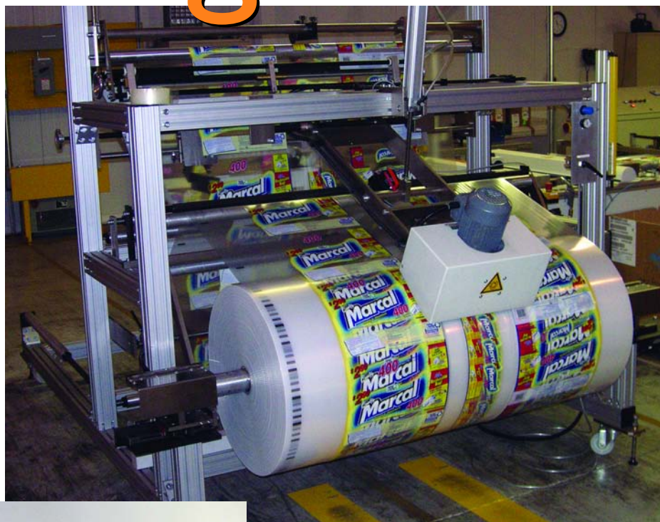
A roll of pre-printed polyethylene film is fed through a Hettler Maschinen FK2000 machine to produce drawstring bags for the U.S.-based paper-napkins manufacturer Marcal Paper Mills.
